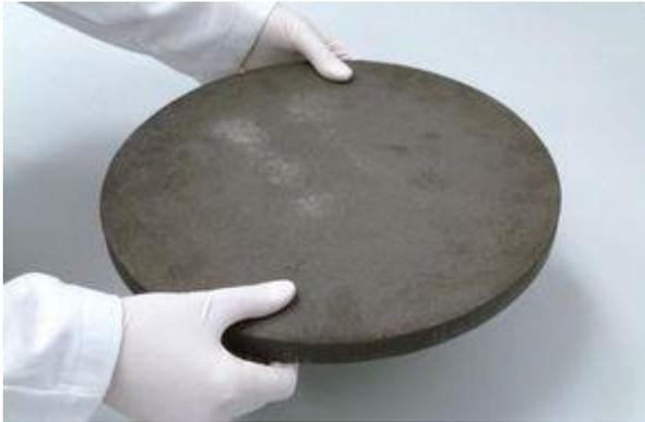
Disk of Mg hydride (up to 600 g of H<sub>2</sub>)
